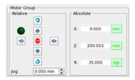
X (sample stage) = Horizontal. The range of this motor is +/- 10 mm.
