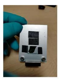
For example, when preparing a powder sample on carbon tape (5.0 x 5.0 mm), use a tool with flat and smooth surface to press on sample surface. For a bulk sample, its surface should be polished.
